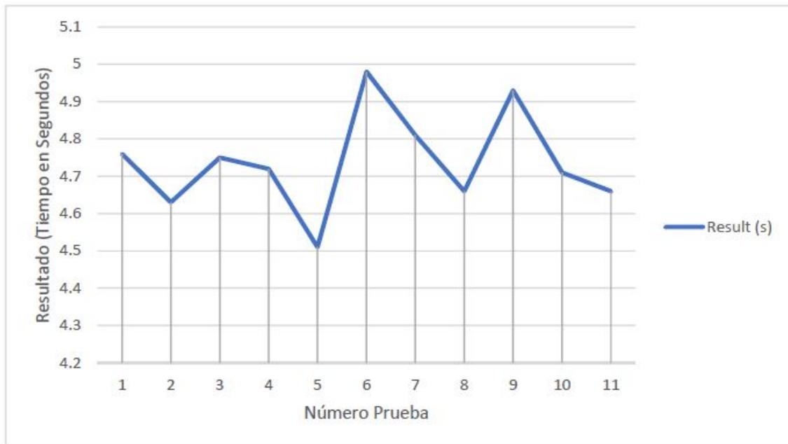
As we can observe the best results was obtained in test five with a result of 4.51 seconds spent performing the calculations of the benchmark. Also, we can observe that the worst performance was obtained with test six which has a result of 4.98 seconds. It is worth a mention that both test five and six have the same values except for the timeslice value. Then we can conclude that in this case a smaller value on the timeslice can have an impact on performance.
